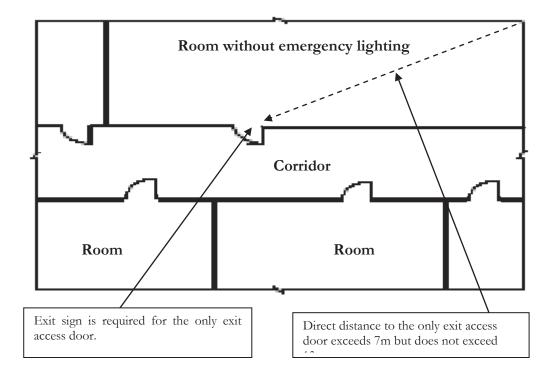
e. When the wall of a room without emergency lighting comprises of not less than 50% glazing and is facing a corridor (with emergency lighting) or external of a building, exit sign over the only exit access door is not required if the furthest point in the room to the exit access door does not exceed 13m
