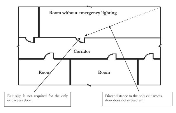
ii. If the direct distance from the furthest point in the room to the only exit access door exceeds 7m but does not exceed 13m, exit sign shall be provided over the door. Alternatively, the room can be provided with emergency lighting
