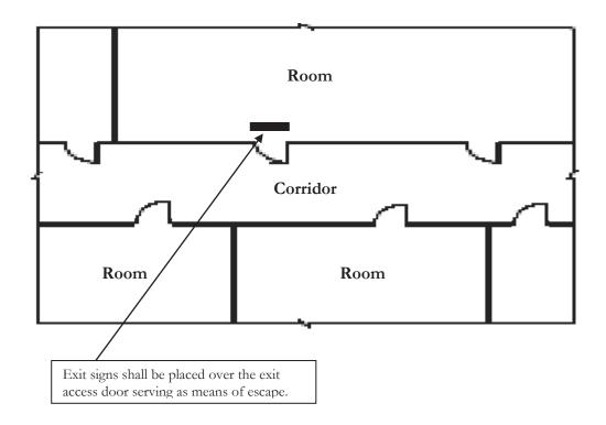
b. In a room provided with emergency lighting and where the line of sight to the exit access door is obstructed, directional sign shall be provided. When only one exit access door is provided in the room, exit sign is not required at the door
