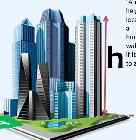
"A distance more than one and a half the height of the building is recommended for locating the AA, or alternately, it can be in a protected area shielded from the burning building by a fire barrier or fire wall, or it may be in an adjacent building if it offers sufficient protection and is able to accommodate the evacuees"
