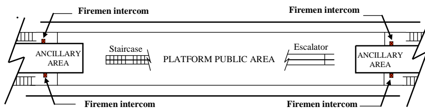
Locations of firemen intercom at platform level
